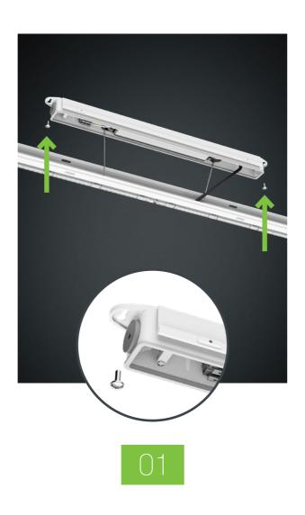
Attach the mounting box to the ceiling using two screws.
